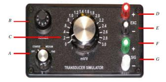
\*The Vernier is included as a diagnostic and setup tool, for example to simulate reaching setpoints in a batching application dry run. It is not designed to have the high accuracy as is specified for the rotary selection knob.
